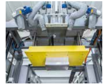
Upper mould plate (for pressure forming) Piano stampo superiore (per pressure forming)
